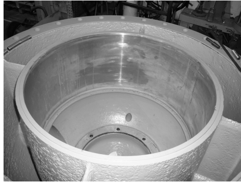
Fig 11: Refurbished plunger cavity
