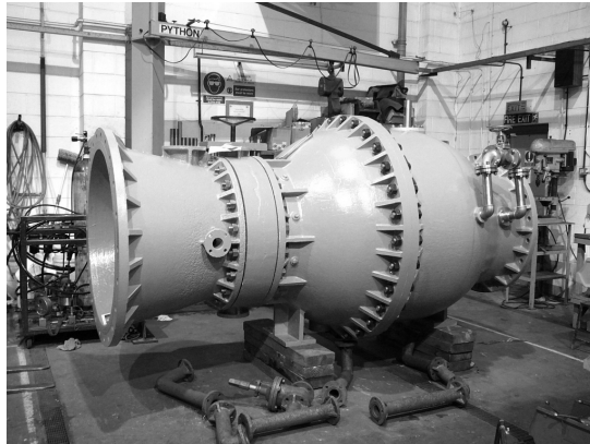
Fig 13: Complete refurbished valve.
