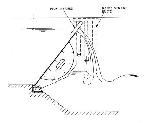
Figure 8. Venting the overflow of a gate
