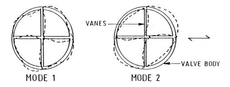
Figure 11. Possible vibration modes of hollow cone valves (after Mercer)
