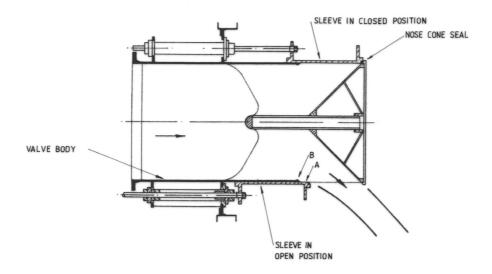
Figure 10. Hollow cone valve
