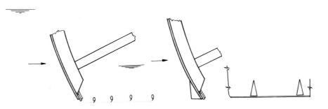
Figure 6. Regular eddy shedding at the bottom of radial gate
