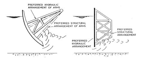
Figure 9. Preferred hydraulic structural arrangement of a gate subject to drowned discharge
