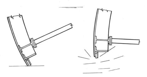
Figure 5. Structural reinforcement of the bottom of a radial gate which can cause flow reattachment when the gate is raised
