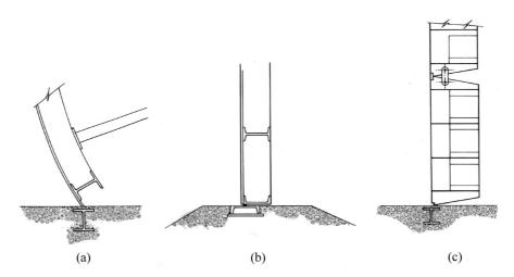
Figure 4. Unsuitable arrangement of structural stiffening members at the bottom section of gates
