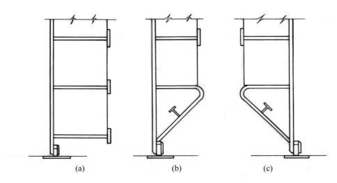
Figure 3. Structural reinforcement of gate bottoms
